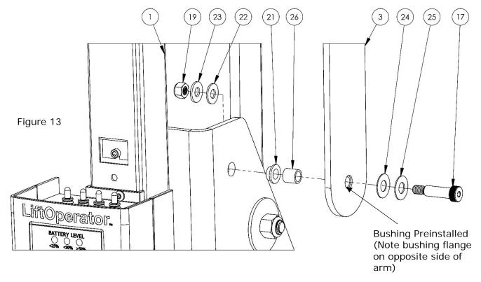
19. Tighten bolt and lock nut until snug; then back off 1/2 rotation.
