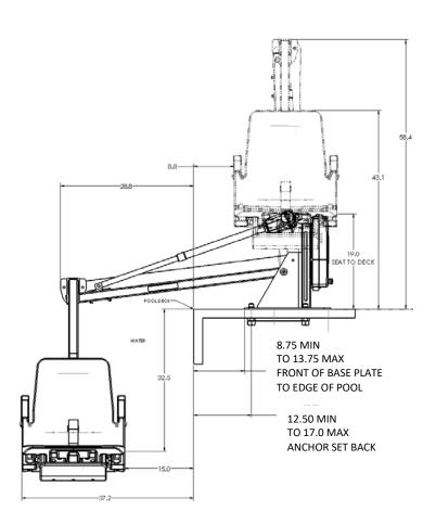
MINIMUM DISTANCE BETWEEN FLUSH DECK ANCHORS AND EDGE OF CONCRETE SLAB SHALL NOT BE LESS THAN FOUR (4) INCHES.
