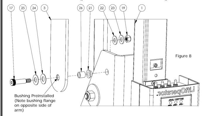
12. Tighten bolt and lock nut until snug; then back off 1/2 rotation.
